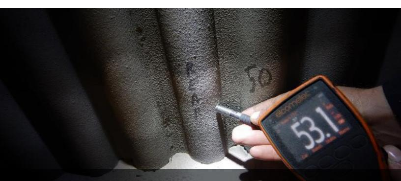
Figure 2. CFB Combustor boiler tubes protected with HVTS Cladding at the tube and refractory interface
