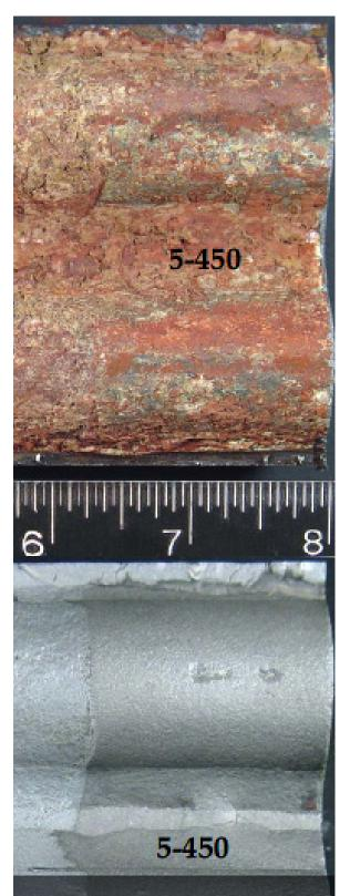
Figure 3. Zimmer EPRI Study, above photo as received, below photo after light sandblasting to reveal HVTS Cladding has protected the tube from fireside corrosion (no wall loss)
