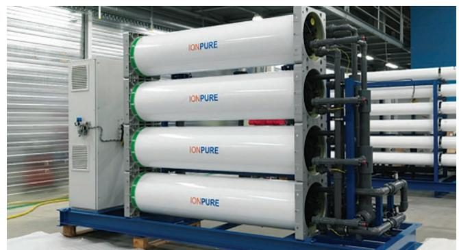
**Figure 4** 264 gpm (60 m<sup>3</sup>/h) CEDI system using stacked-disk modules
