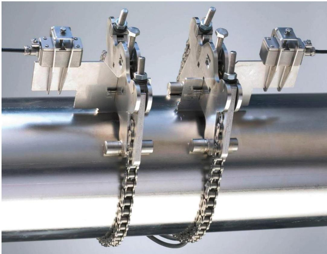
*FLEXIM’s WaveInjector mounting method is designed to allow the transducer to be mounted at a safe distance from the pipe to protect against heat damage while still providing accurate measurements.*
